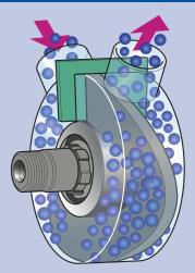
A single sinusoidal rotor in the pump creates four evenly sized chambers as it rotates within the pump. Fluid is "pulled" through the inlet on the suction side into each chamber in turn. As each chamber rotates, it contracts, closes and finally discharges fluid through the outlet port. At the same time, the opposite chamber opens to draw in more fluid. The result is a perfectly smooth flow, free of any pulsation.
